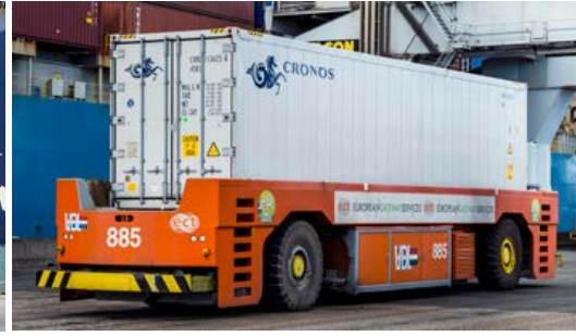
Figuur 7: Automated Guided vehicle (AGV) (Transport-online, 2013)
